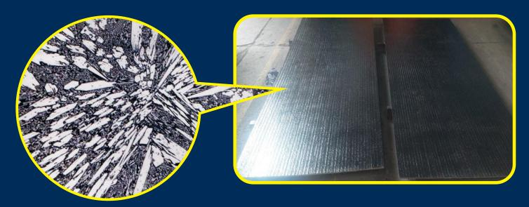
Remarks: Micro-structure shows the Primary Chromium Carbides & Eutectic Carbides with Austenite & Martensite
